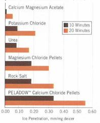
A melt volume comparison of PELADOW™ Calcium Chloride Pellets with other products at 5°F (-15°C) illustrates the greater effectiveness of calcium chloride when melting ice at low temperatures. PELADOW™ melts ice up to three times faster than competing materials.
